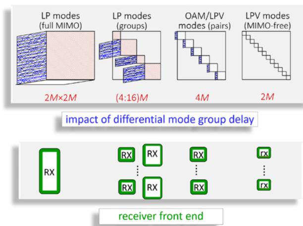
Fig. 1 Illustration of MIMO processing complexity (upper section) and receiver front end complexity (lower section) for various MDM solutions.
