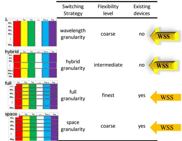
Fig. 2 WDM-MDM switching architectures and their attributes; full and partial MIMO systems compatible with wavelength and hybrid architectures, respectively;  $2 \times 2$  MIMO and MIMO-free compatible with all architectures
