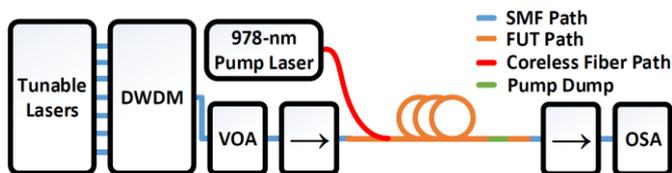
Fig. 3 Experimental setup used to measure gain and noise figure.
