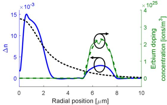
Fig. 2 Measured refractive index profile  $\Delta n$  (blue), measured (solid green) and fitted (dashed green)  $\text{Er}^{3+}$  doping concentration profile, and calculated mode profile at 1530 nm (dashed black)
