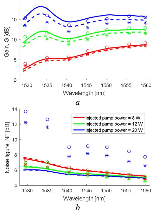
Fig. 4 Simulation/experimental results for the gain, G (a) and noise figure, NF (b) when one core is loaded with signal input power of -23.1 dBm (solid line/circle) and 1.4 dBm (dashed line/asterisk) for injected pump power of 8 W (red), 12 W (green) and 20 W (blue)
