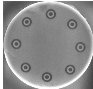
Fig. 1 Cross-section of the 8-core erbium-doped fiber with annular doping in the cladding and with a core-to-core distance of  $38.25 \mu\text{m}$
