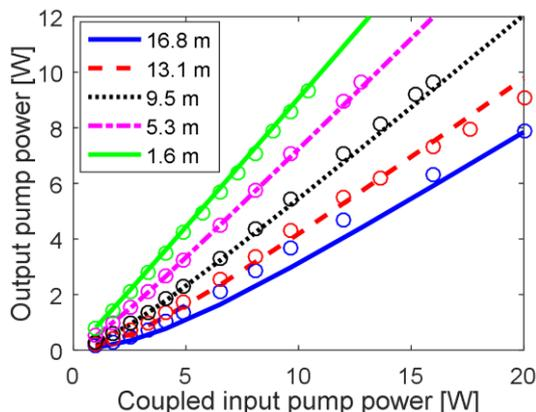
Fig. 5 Experimental (circles) and simulation (lines) results for the output pump power (without any input signals) when the injected pump power is varied between 1 and 20 W and the fiber length is varied between 1.6 m and 16.8 m.
